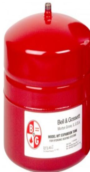
The B&G HFT tank is a non-code small diaphragm tank with a maximum of 100 PSIG working pressure. This tank is used where ASME is not required and the system is a lower system volume. An example is a residential system.
